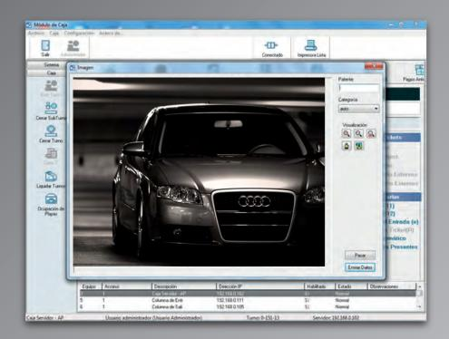
You can also configure the system to send an Alert with the vehicle image to the cashier on every entry, allowing the licence plate and category pre-load before printing the ticket.
